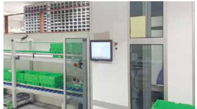
RoboPharma's operating system steers the network of high-speed dispensing robots and integrated tote conveyors so there is no holdup or backup to each hospital ward's mini-pharmacy.
